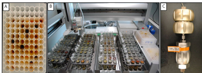
Figure 2. Automated LC-RP C18 system; A) Crude Extracts, B) Gilson 215 System with Custom Racks Holding Genevac Evaporator Racks, C) C18 Reverse Phase Column with Guard.
